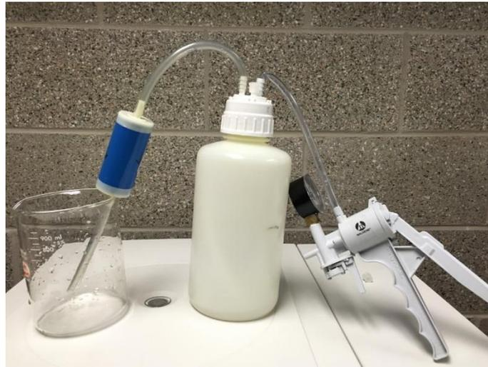
**Figure 1. Pressurizing device for forcing challenge water through the water filter.** A hand pump was used to generate pressure inside the vacuum bottle, which then forced test water through the filter at 5-10 psi.
